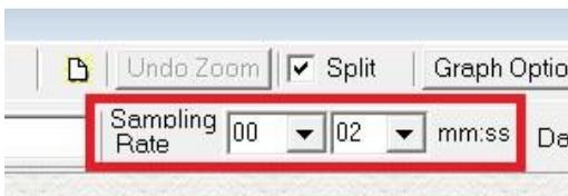
(5) When the connection is successful, click “ **Real Time | run** ” or
