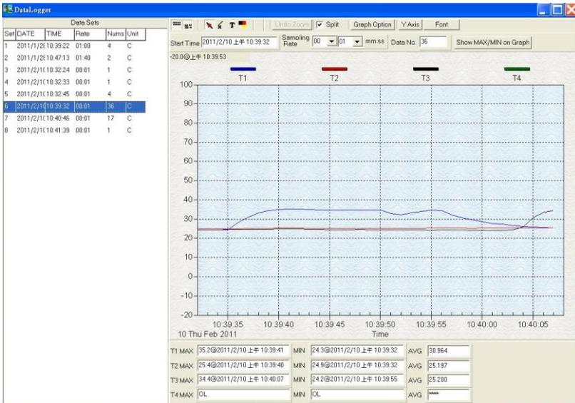
When you have the thermometer connected to PC, select " **DataLogger** " from main menu or click Datalogger icon from tool bar to load recorded data from the meter and there will be a progress indicator to show the loading status. If error occurs, just click " **DataLogger icon** " again.
