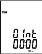
(3) Fig.3 Set interval time for data logging.
